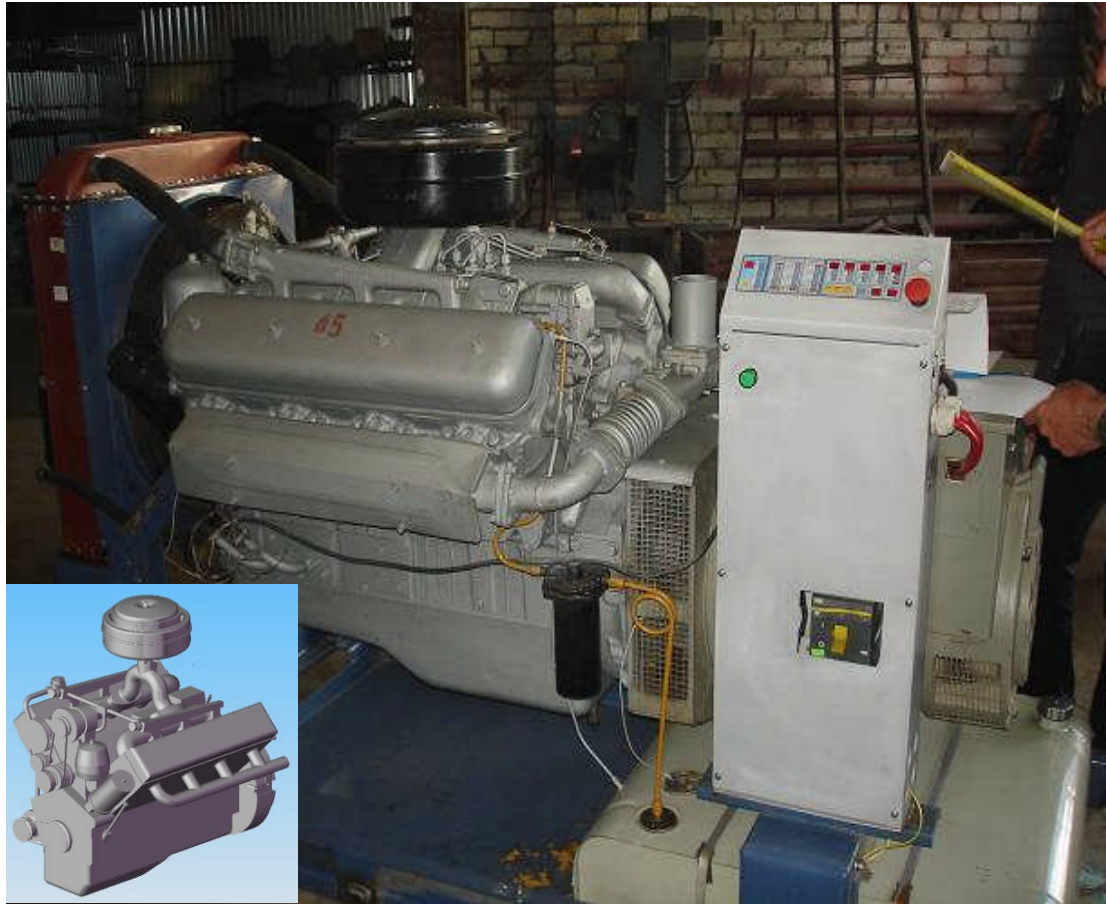
Tested Engine at NAMI with an electric power generator.
