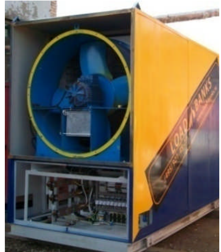
View of the 120 kWt load testing bench for testing the engine with the generator
